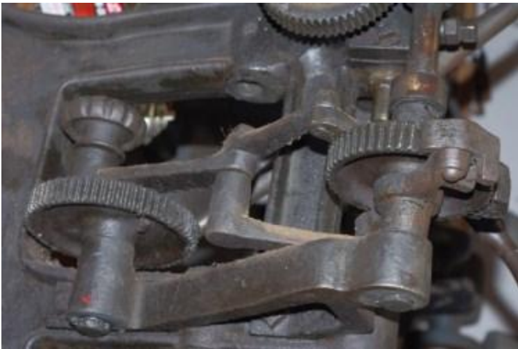
Auto feed assembly, looking from below, rear to left
