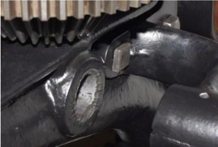
Support bracket attached with 'flat' head bolt in front
