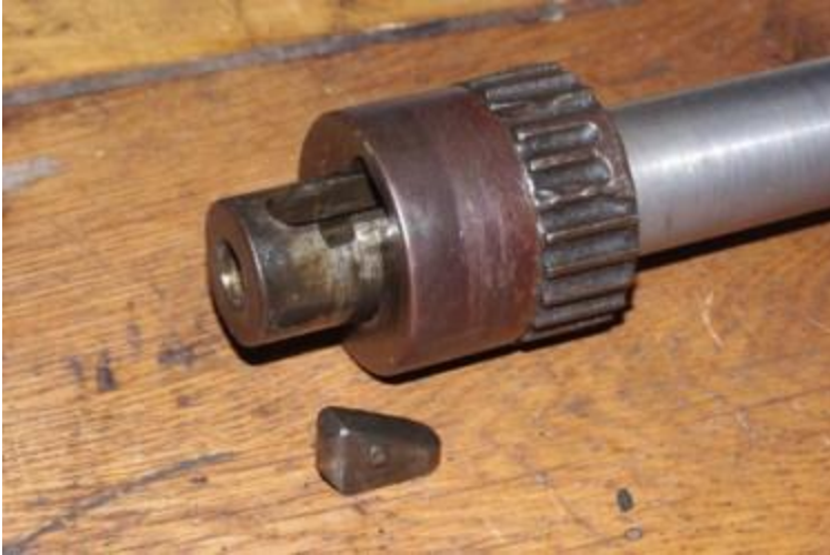
Pressure wedge removed and sitting in correct orientation
