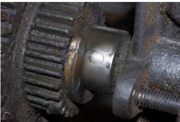
Pin locking bevel gear to flywheel shaft exposed by sliding double gear down
