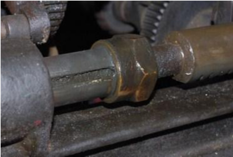
Brass nut attaching feed sleeve and mandrel before disassembly
