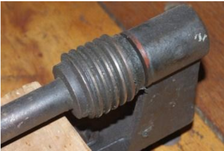
Upper bracket/arbor bearing with worm gear and fiber washer
