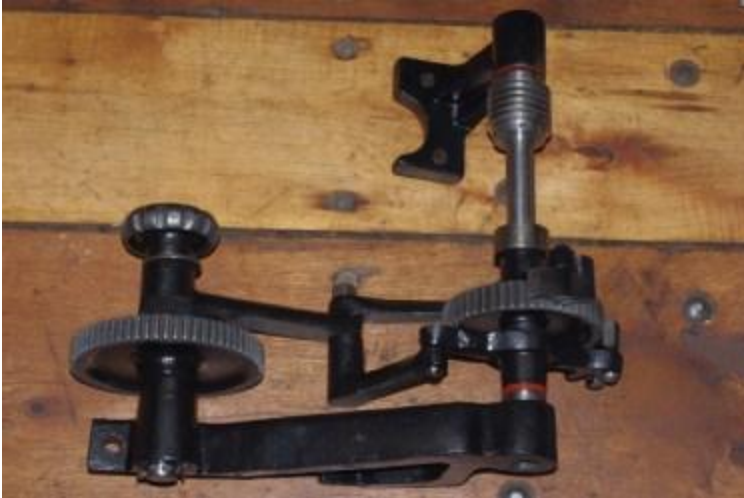
Reassembled auto-feed assembly
