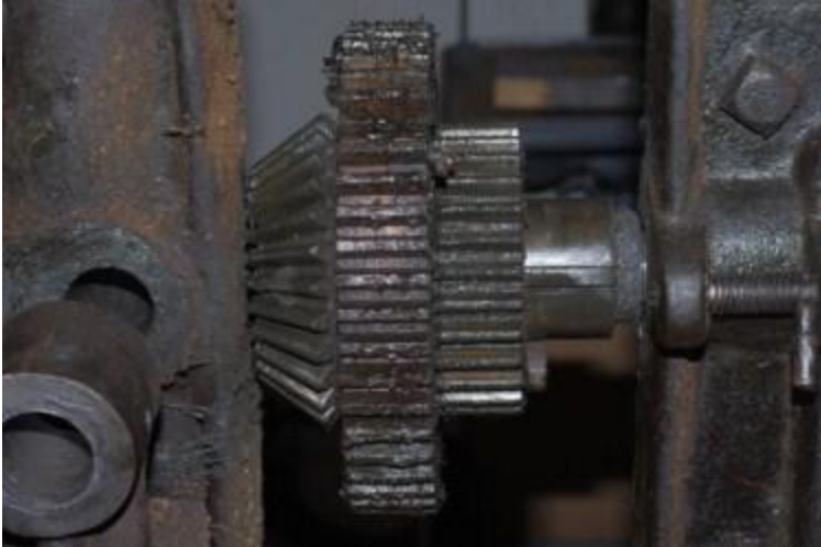
Bevel gear with double gear in lower position
