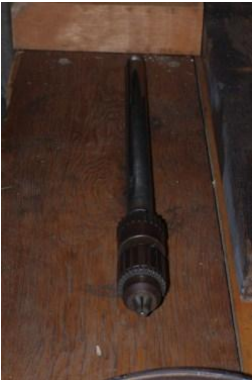
Mandrel with original 'safety chuck' holding Jacob's chuck
