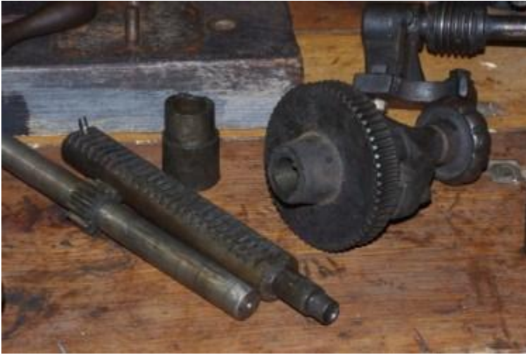
Pinion feed shaft, feed shaft sleeve and clutch assembly removed
