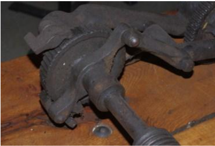
Auto feed assembly viewed from above right
