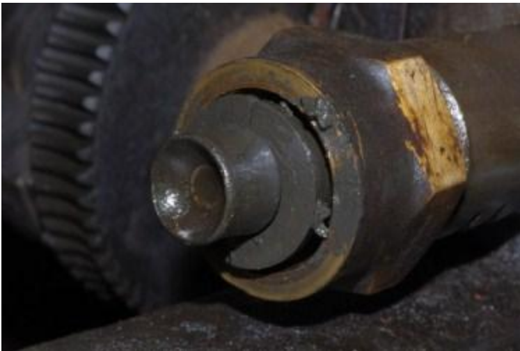
Bottom end of feed sleeve with split washer in place
