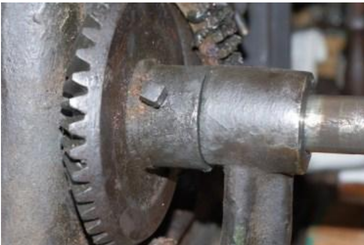
Large bevel gear on crank shaft between frame and support bracket
