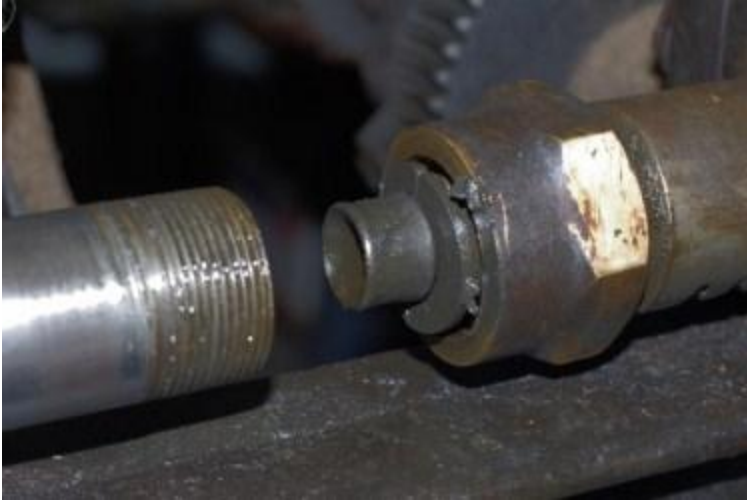
Brass nut loosened from mandrel
