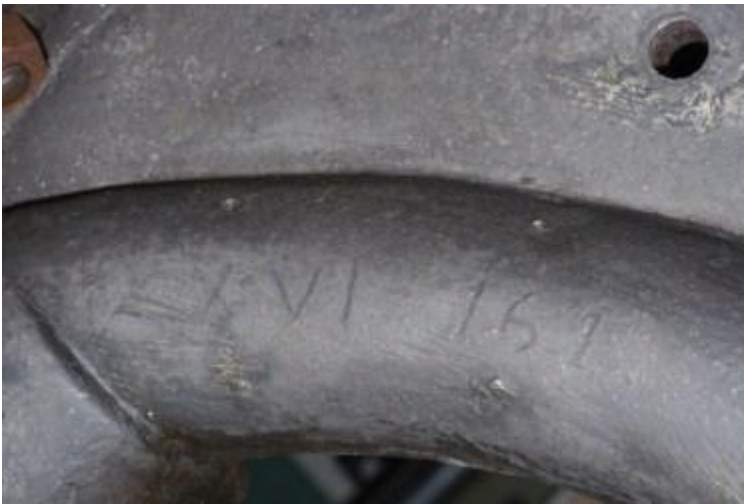
Casting marks on frame
