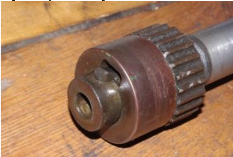
Safety chuck with lower collar slid upwards to expose pressure wedge
