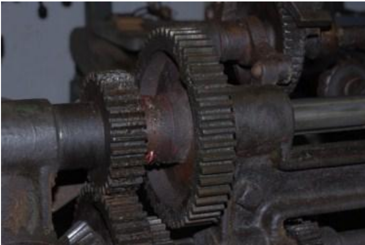
Mandrel gears in place before disassembly
