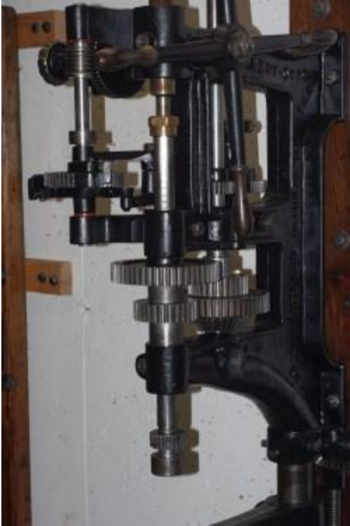
Mandrel shaft and gears replaced viewed from right
