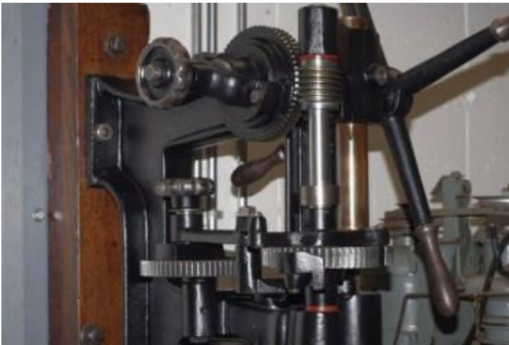
Auto-feed assembly replaced on machine
