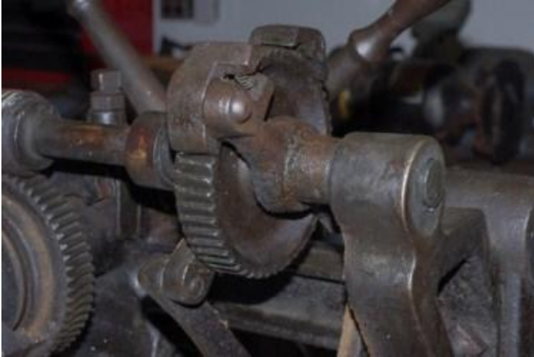
Ratchet gear assembly
