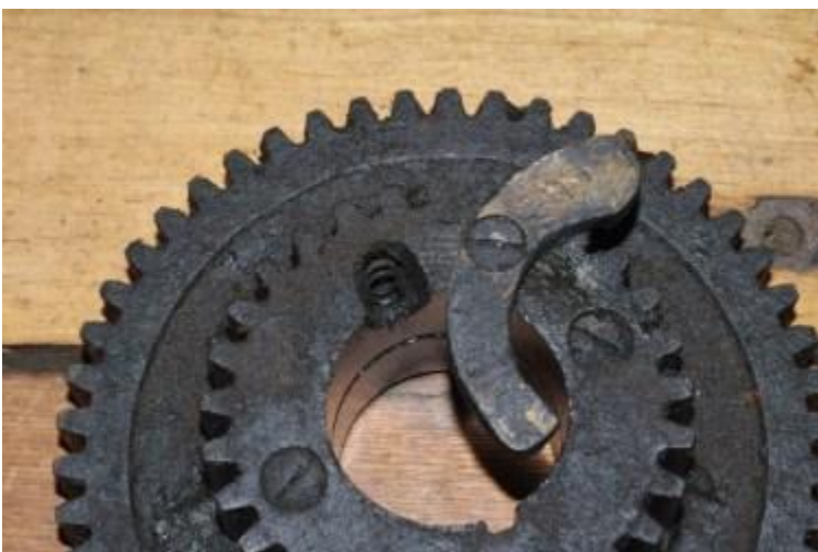
Brass gear release latch moved to expose spring
