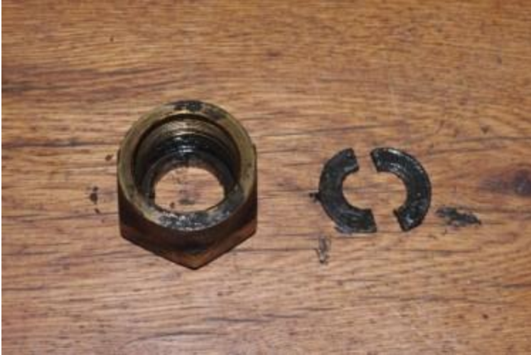
Large brass nut with left hand thread and split washer
