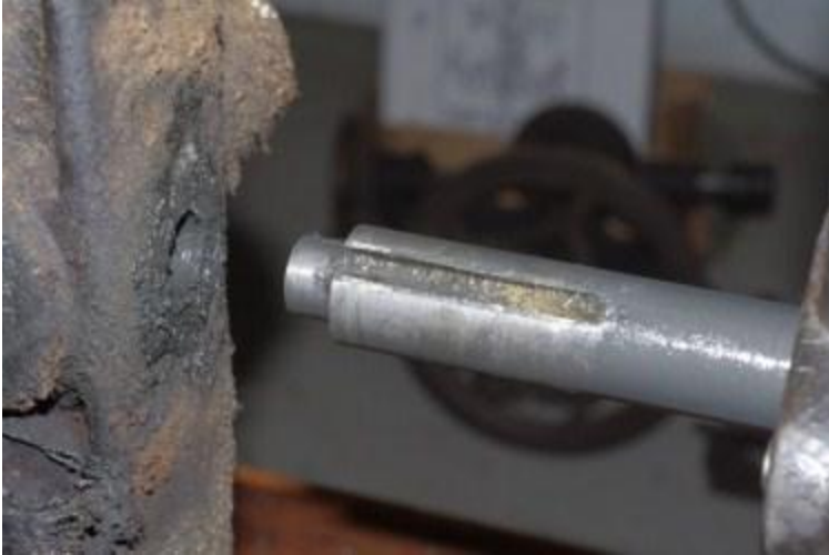
Bottom of flywheel shaft with machine key groove for bevel gear
