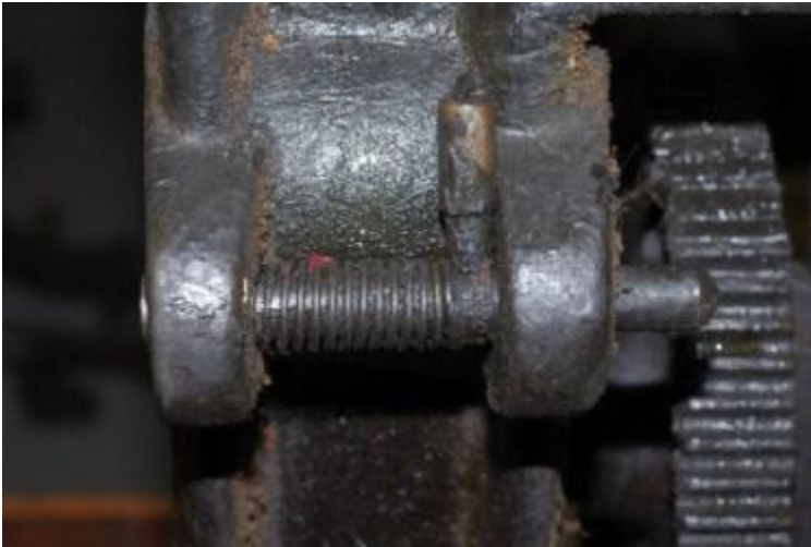
Gear release pin
