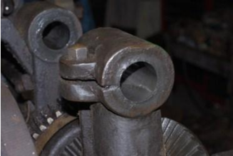
Lower mandrel bearing and tension bolt
