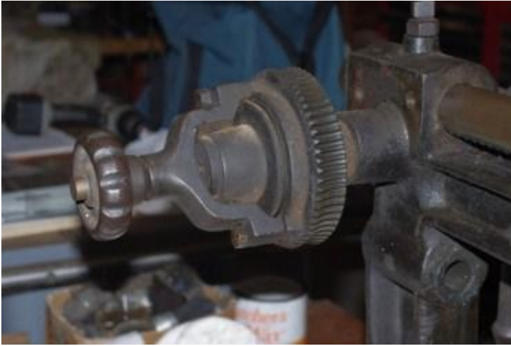
Clutch assembly and spiral feed gear
