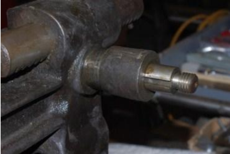
Pinion shaft sleeve partly driven out from frame. Groove in shaft is for handle.
