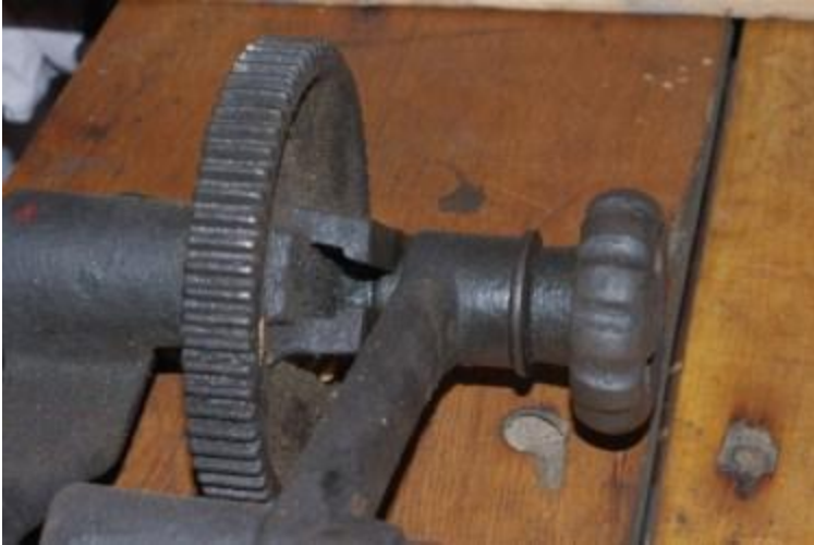
Feed rate adjustable bolt with handle in slot on large feed gear
