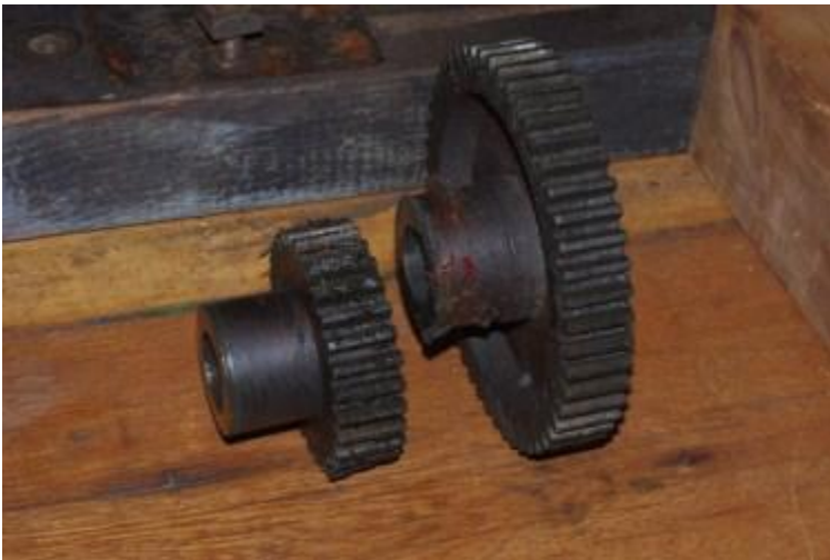
Gears from mandrel shaft removed and in correct orientation
