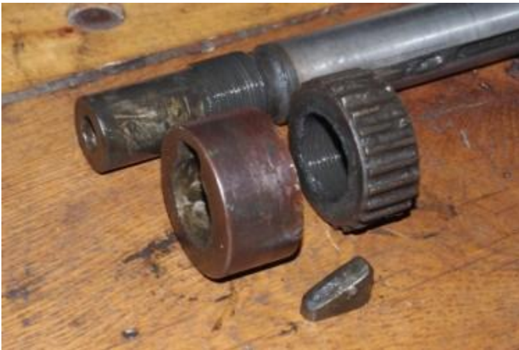
Safety chuck removed (wedge is sitting backwards)
