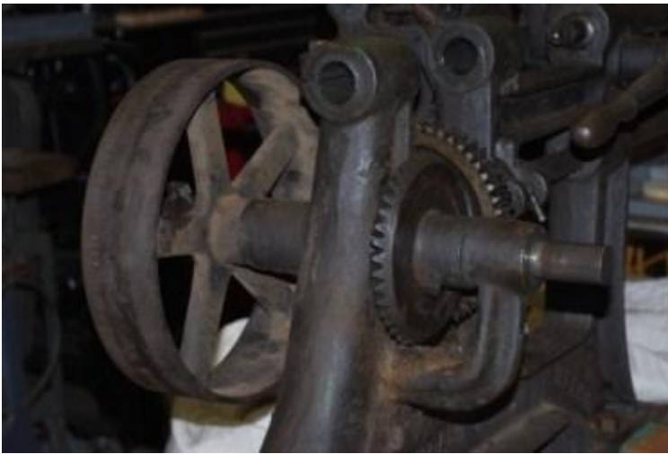
Crank/pulley shaft with bevel gear in place
