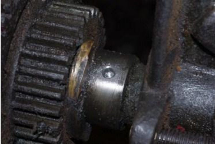
Outer aspect of pin drilled out to remove deformity and allow removal
