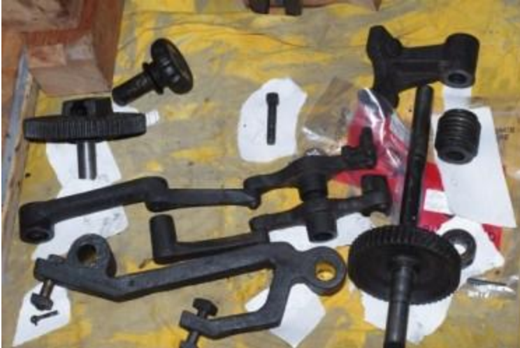
Auto feed assembly taken apart, in approximately correct orientation, parts numbered to correlate with numbered notes
