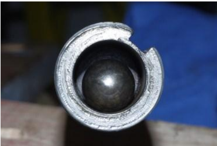
Ball bearing in top of mandrel shaft
