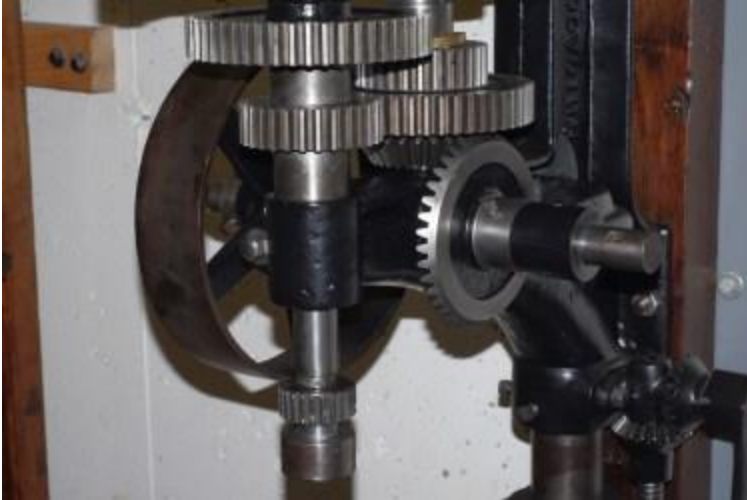
Crank shaft, bevel gear, support bracket and pulley replaced. Viewed from right
