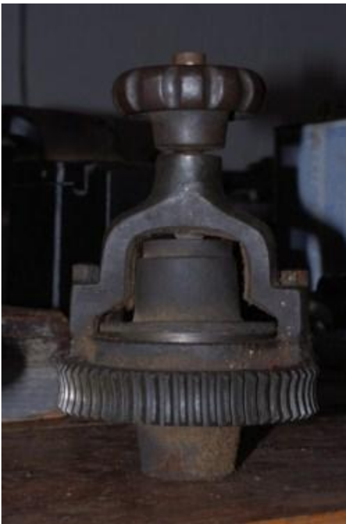
Clutch assembly and spiral gear removed
