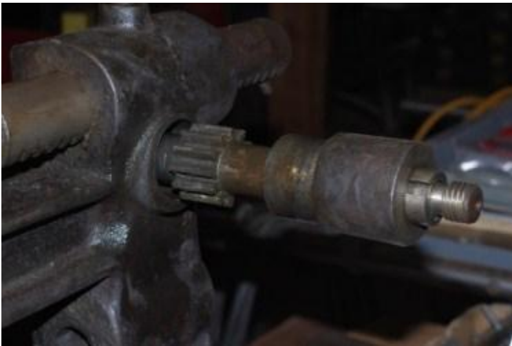
Pinion shaft with gear, with sleeve removed from frame
