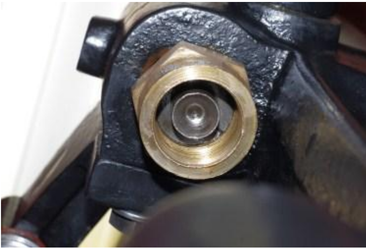
Large brass nut held in place by split washer in groove of pinion rack sleeve
