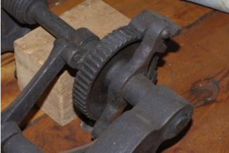
Arbor with long feed arm above gear and short feed arm and bracket below gear
