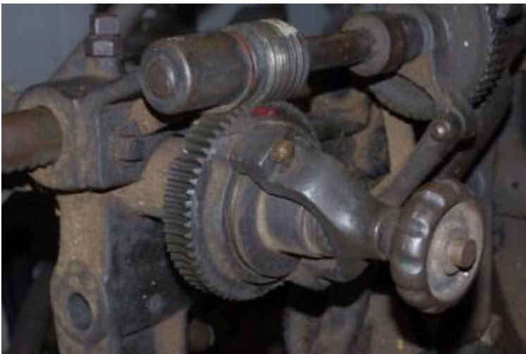
Worm gear with spiral feed gear, top of drill press to left
