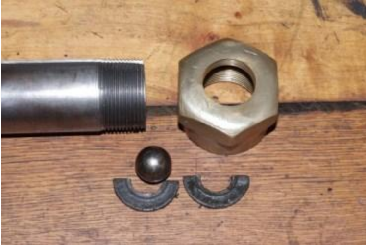
Top of mandrel shaft with large brass nut, split washer and ball bearing
