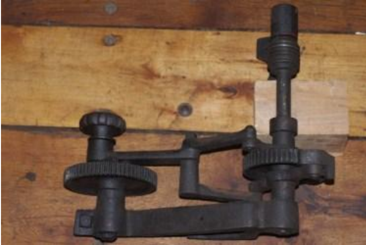
Auto feed assembly intact
