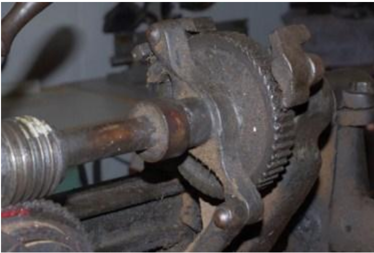
Worm gear shaft passing through ratchet feed gear
