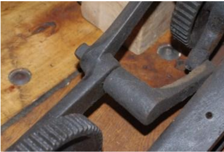
Long and short feed arms attached by bolt at pivot point
