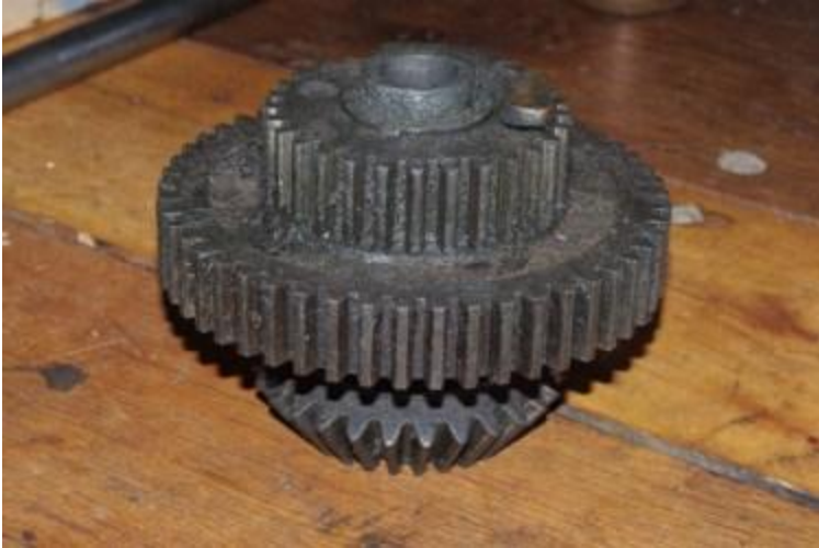
Fly wheel shaft double gear in upper position on bevel gear
