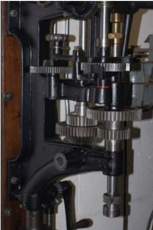
Mandrel shaft replaced viewed from left
