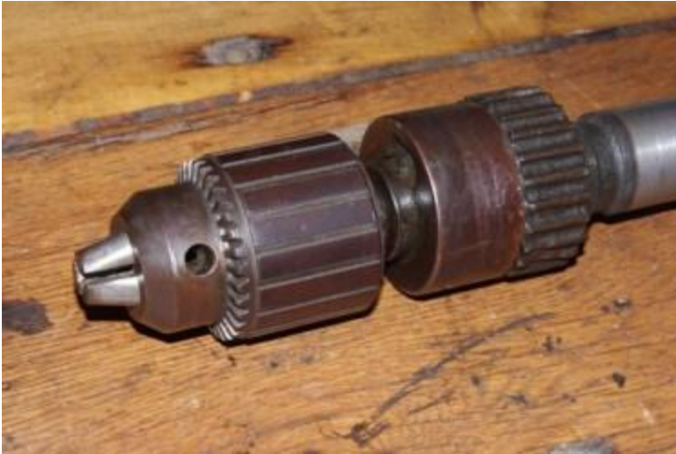
Original 'safety chuck' holding newer Jacob's chuck with adator
