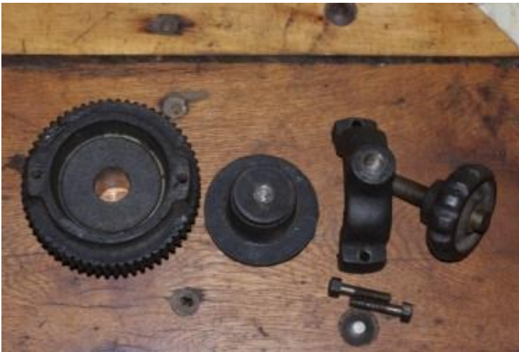
Clutch assembly taken apart
