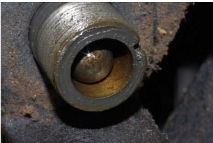
Top end of mandrel with ball bearing
