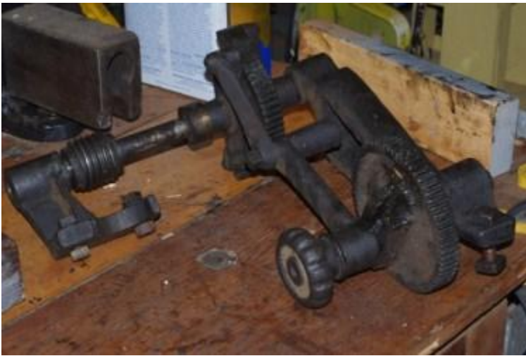
Auto feed assembly removed
