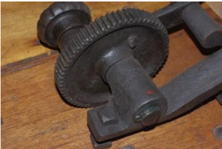
Large feed gear with attached arbor in rear of lower bracket
