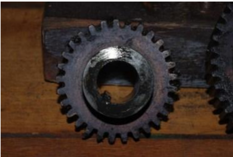
Gear with machine key
