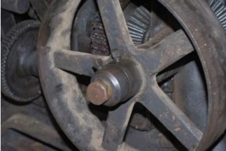
Drive pulley with collar
