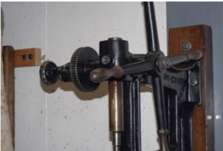
Feed rack replaced, viewed from right
