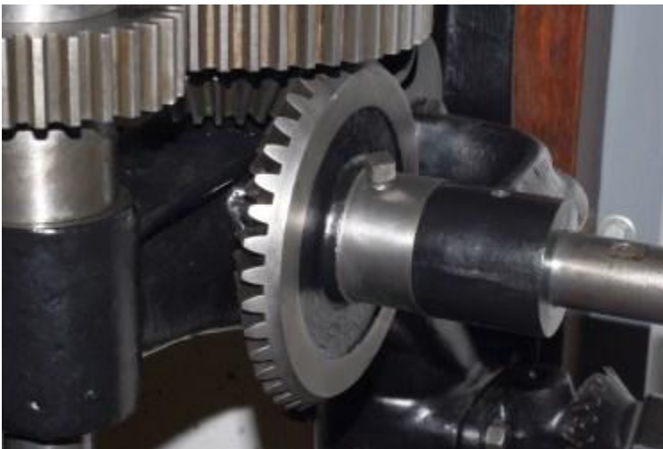
Shaft and bevel gear replaced
