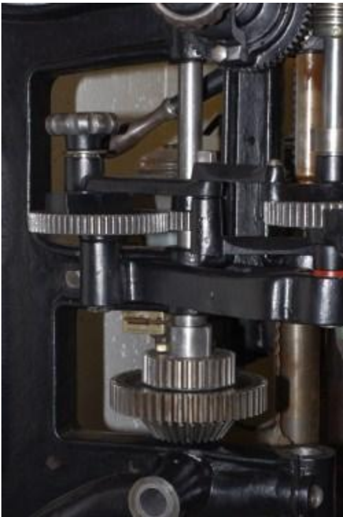
Mandrel shaft and gears replaced view from left
