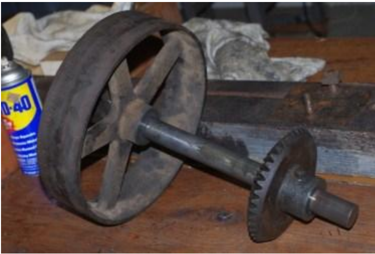
Crank shaft, pulley and bevel gear after removal
