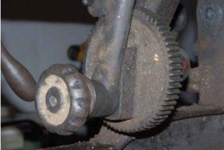
Large feed gear with 'eccentric' feed rate adjustment bolt
