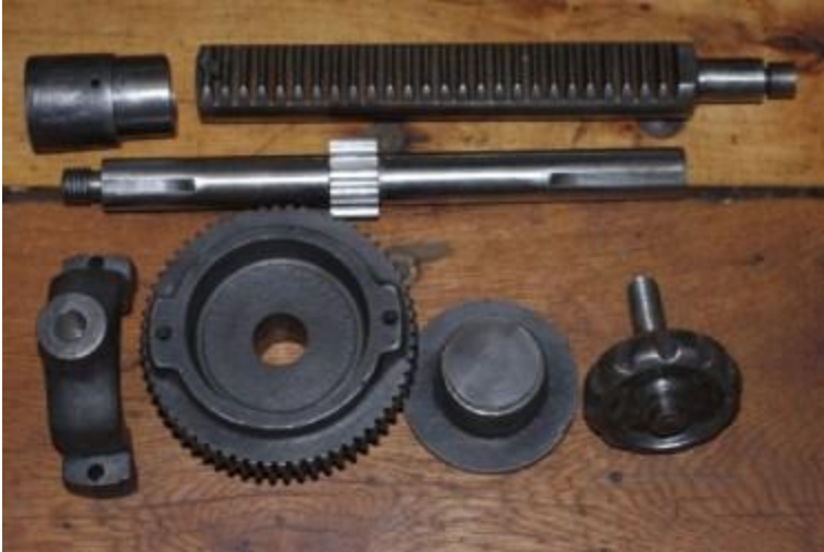
Feed shaft, rack and clutch assembly. Handle not shown.
