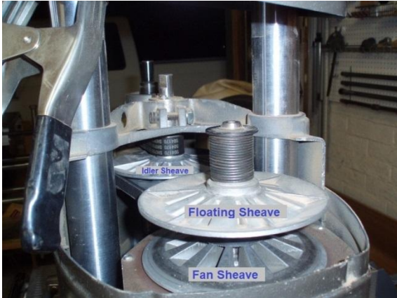
Low Speed Sheave Positions - Photo credits - Dusty post #174149
