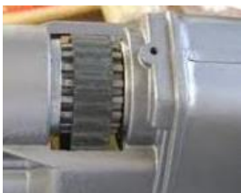
The earlier Gilmer Drive Sleeve Assembly mounted in the Headstock viewed with the Belt Cover removed. An anomaly on this photo may first escape you. 1960 Goldie Headstock introduced the Poly-V Belt system. The Gray Mark V with the Gilmer Drive never came that way from the factory. This headstock was actually repainted by Jerry. A Gilmer Drive in a newer Headstock could also be done. Grey doesn't mean newer any more than Green or Gold always mean older. Tribute re-painting occurs on Headstocks that were replaced, or an original Greenie or Goldie vintage unit may be upgraded internally with new parts. Photo credit Jerry in 'Shopsmith Mark V Restoration blog' at Lumberjocks.com
