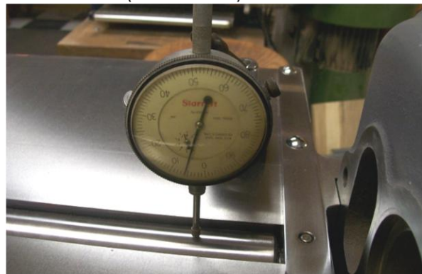
Checking Idler Roller height adjustment across bed
