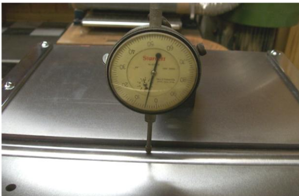
Checking Idler Roller height adjustment
