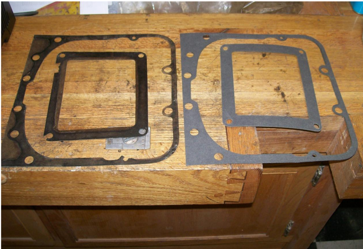
Replacement gaskets made using the originals as patterns
