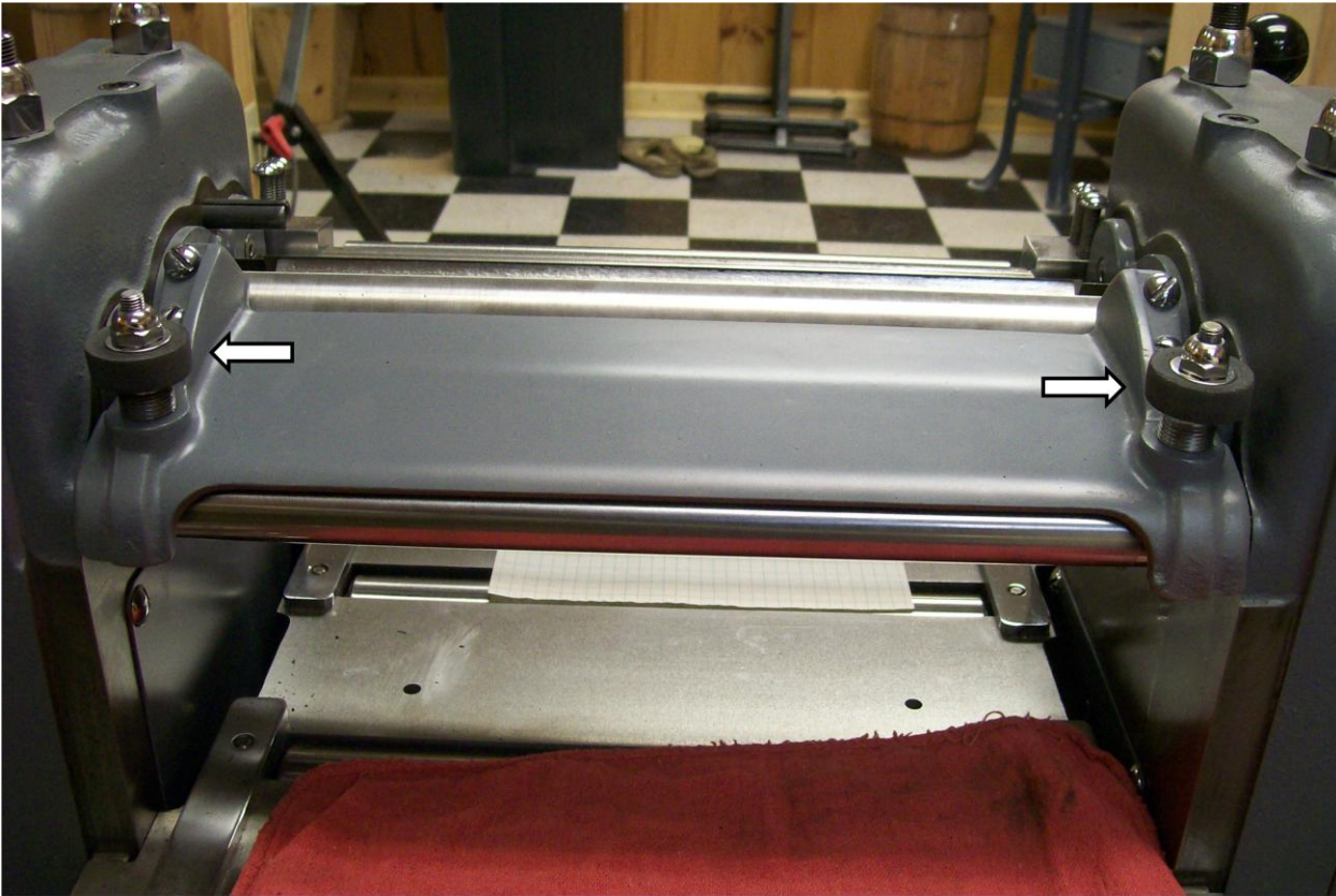
Pressure bar hardware installed
