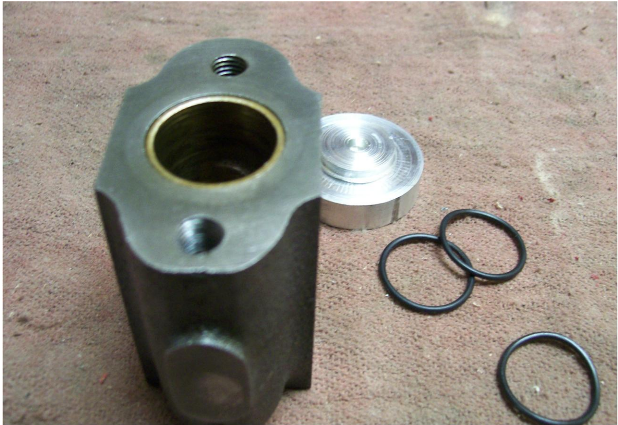
Guide Block with "O" Rings and Recessing Jig
