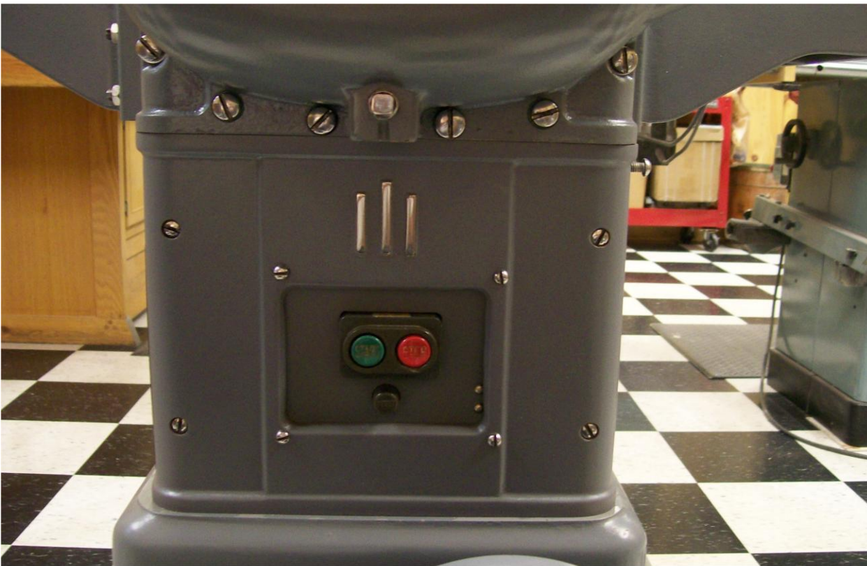
Motor Starter Cover installed.
