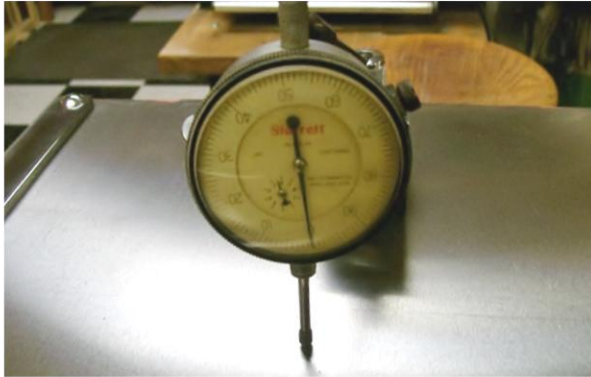
Setting dial indicator for "0" bed height
