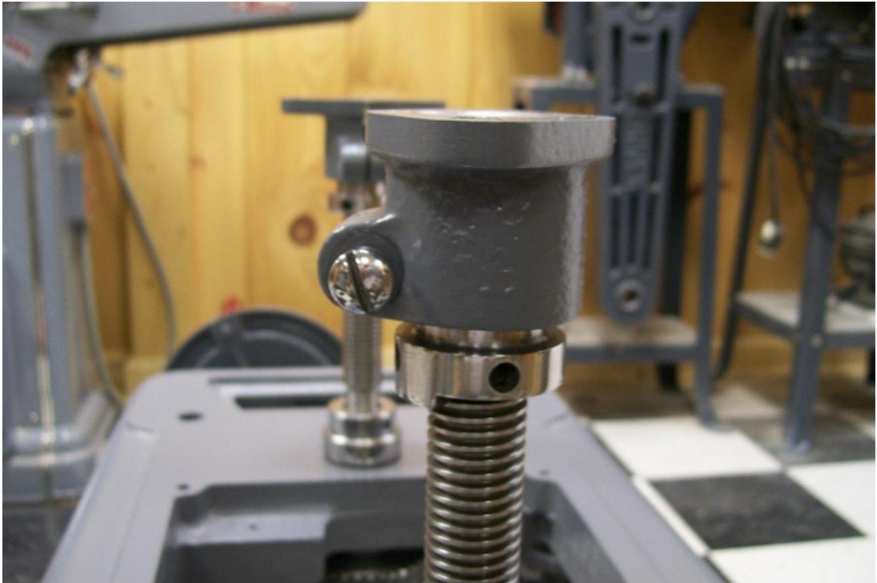
Adjusting nut support and adjusting nut attached to the table elevating screw ready for table
