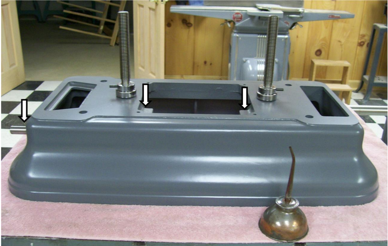
Base with bearings, shaft collars and roll pins installed. Arrows indicate recessed holes in base casting for oiling the raise lower shaft bearings.
