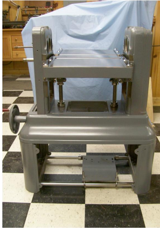
Stand, Base, Table assembly and Support Columns ready for the next phase
