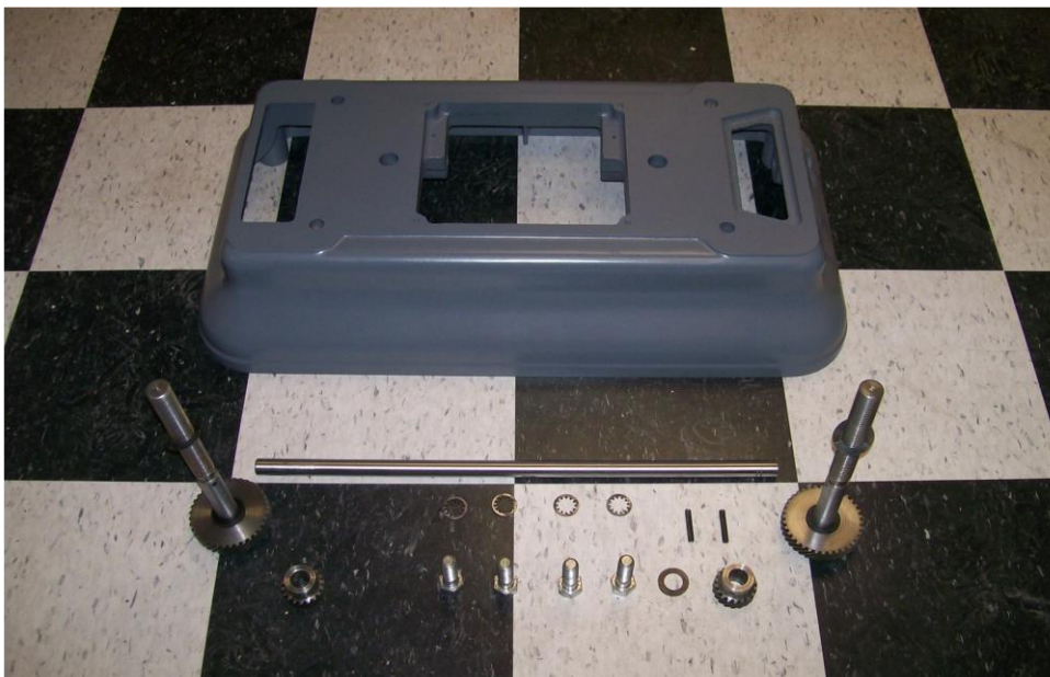
Machine base and raise/lower assembly parts. Not shown are the Spacer Washers.
