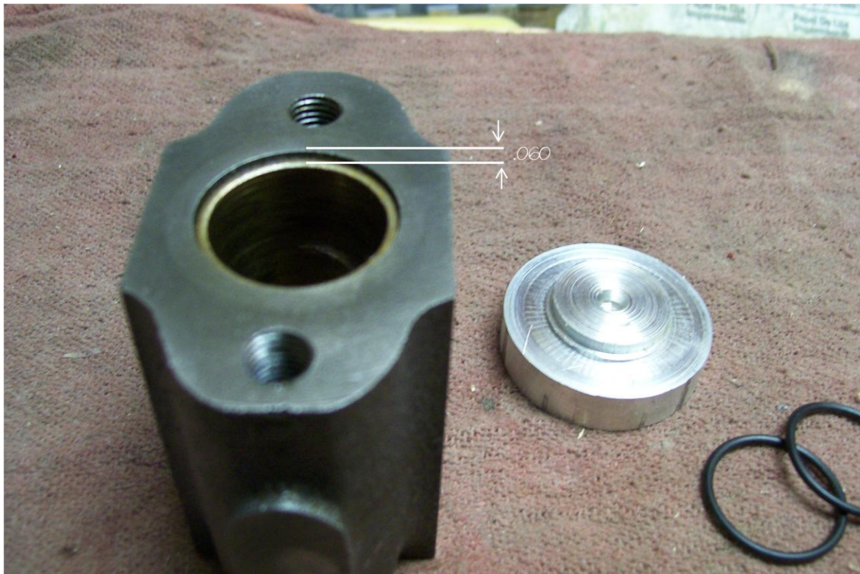
Guide Block with Bearing recessed for "O" Ring
