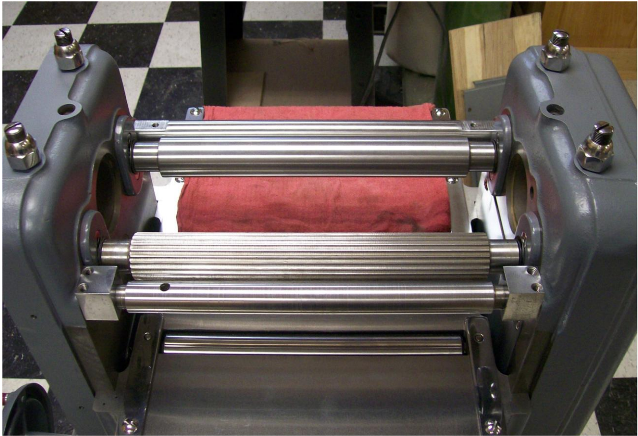
Completed installation of the Infeed/Outfeed Rollers and the Front and Rear Tie Bars.
