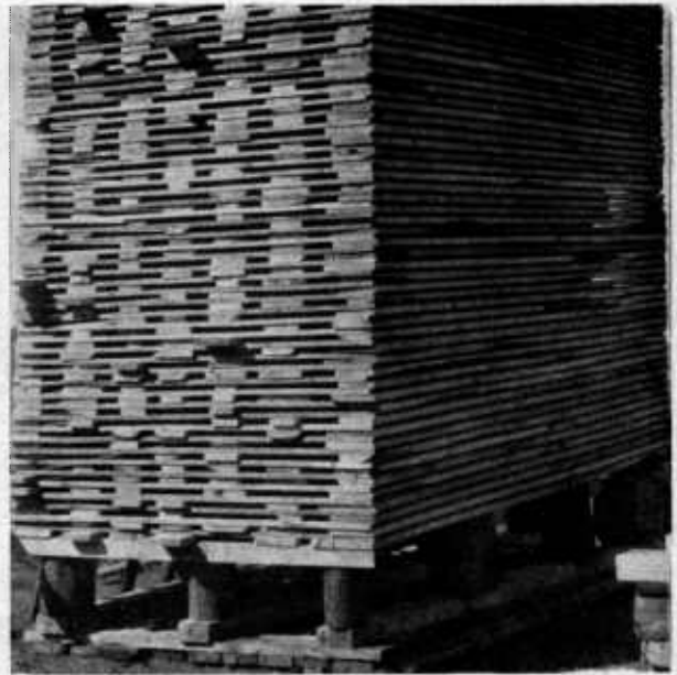
FIGURE 91.—Box pile of random-length hardwoods, supported on sections of logs and cross beams.
