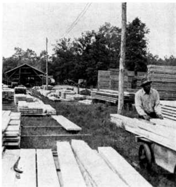
FIGURE 115.—Stacking lumber in unit packages by means of tram car running from rear of mill.
