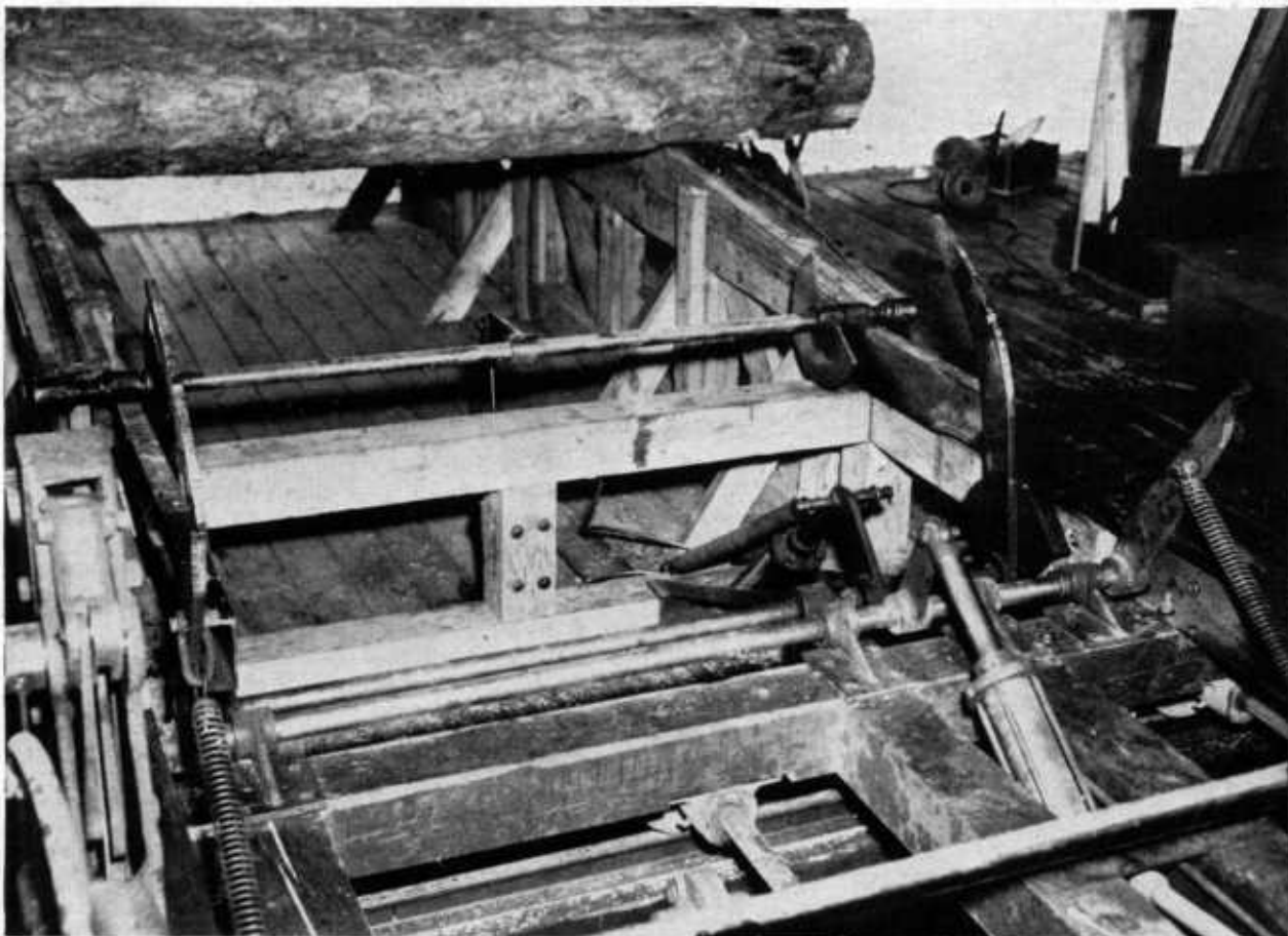
FIGURE 55.—Rocker-arm log turner.
