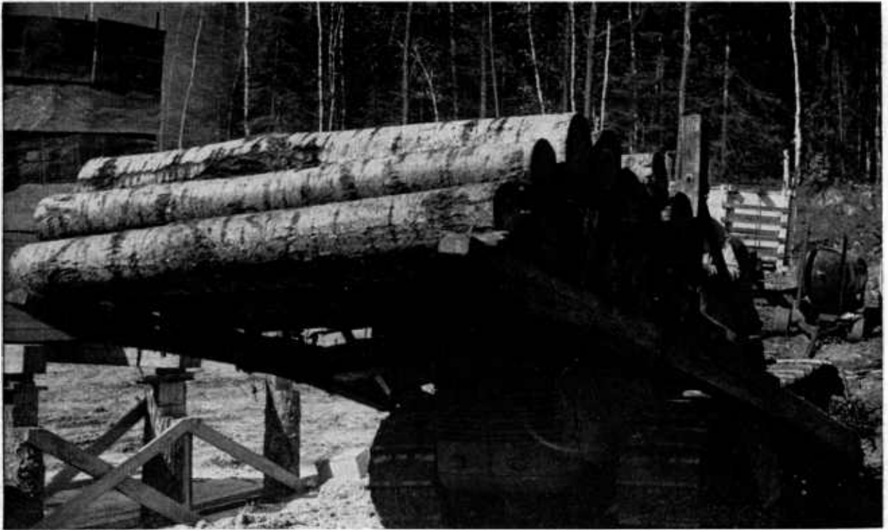
FIGURE 84.—Tractor with rack for yarding logs.
