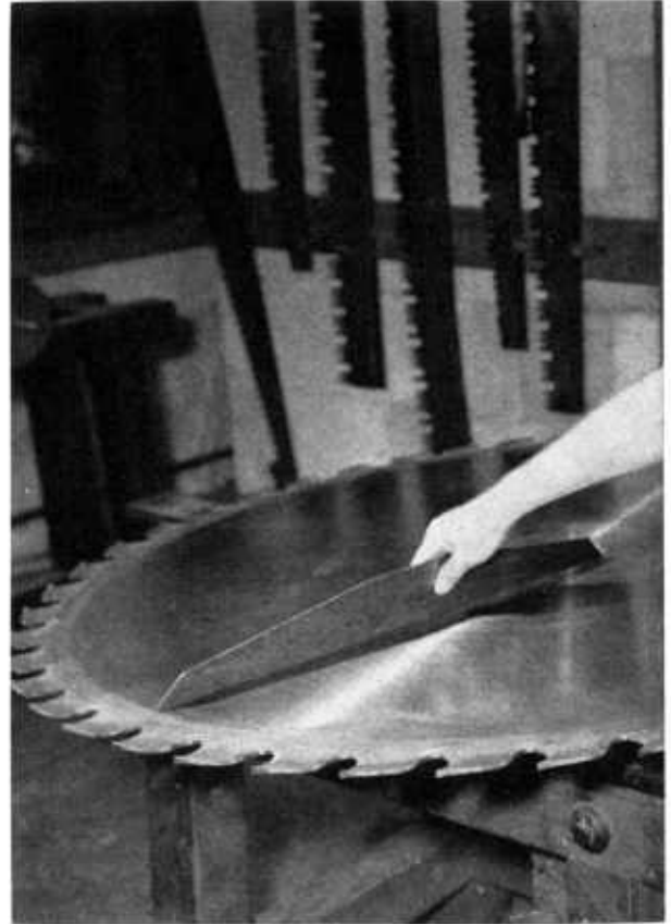
FIGURE 69.—Method of measuring tension in a circular saw.
