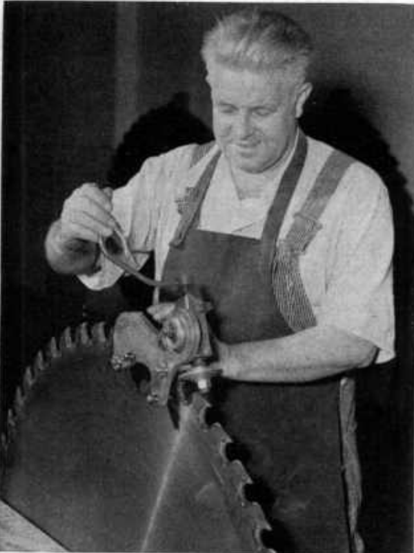
FIGURE 79.—Tooth-sharpening machine using hand-cranked wheel faced with file segments.
