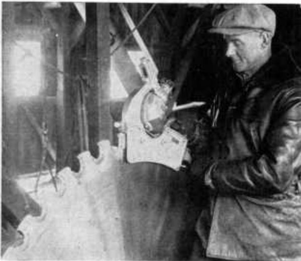
FIGURE 80.—Tooth-sharpening machine with powered emery wheel.
