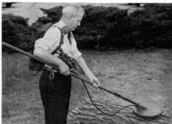
FIGURE 56.—Mine detector used for locating metal in logs.
