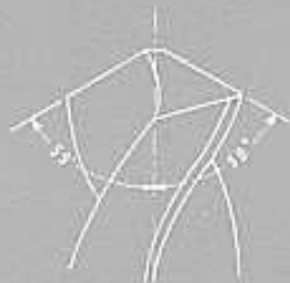
Both lips must be at the same angle
