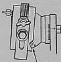
CHASER HOLDING BLOCK SET SO THAT LAND NARROWS PARALLEL WITH CHAMFER
