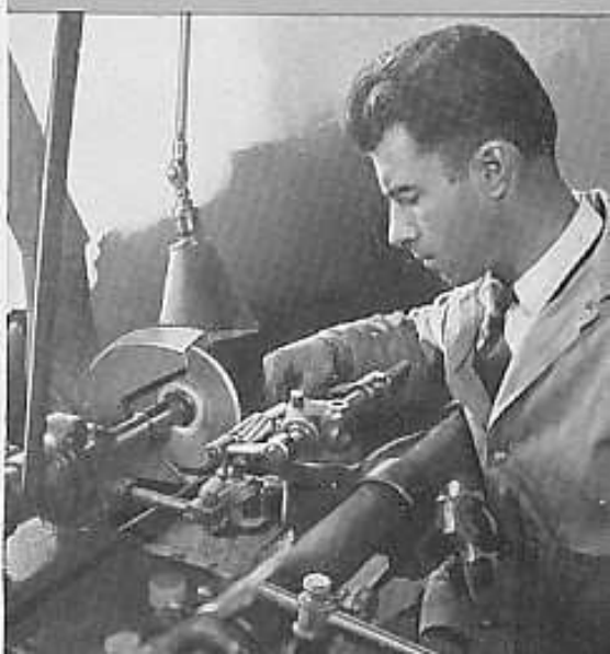
Grinding a Helical Milling Cutter with steep angle of helix
