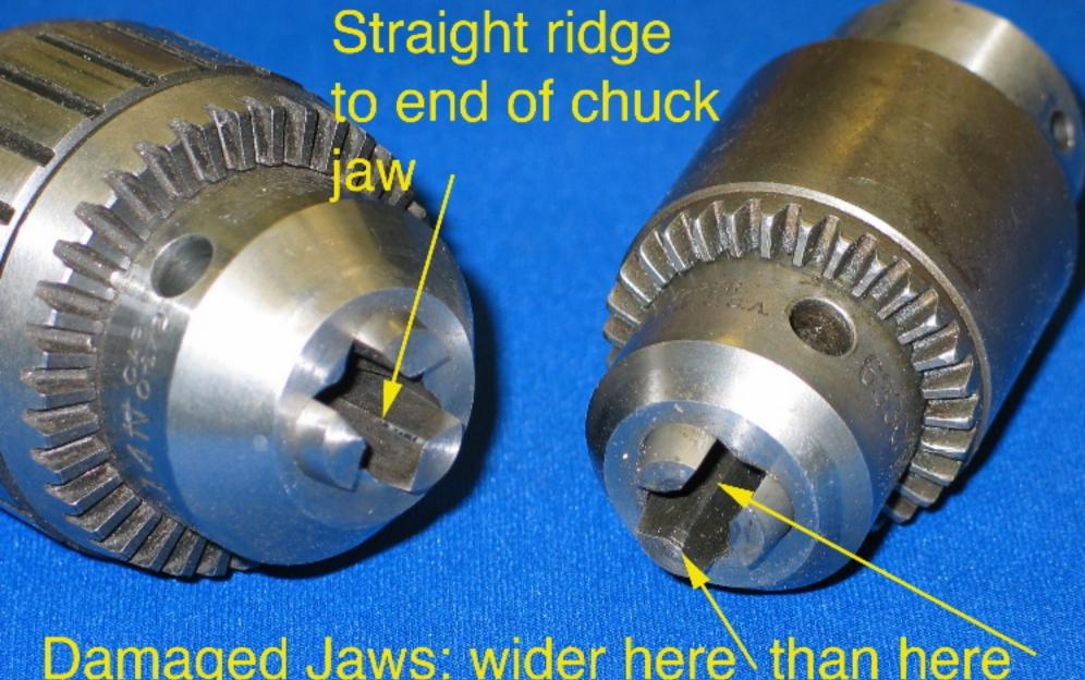
Damaged Jaws: wider here\than here\
