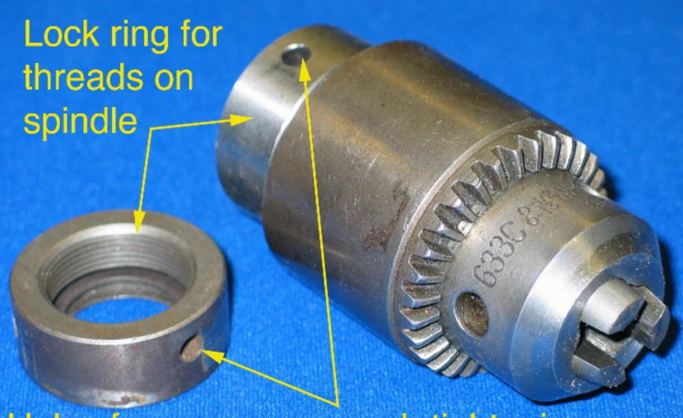
Holes for spanner wrench tightening and loosening the chuck on the spindle
