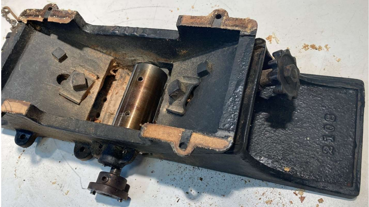
The underside of the jointer, after removal from its baseplate.
