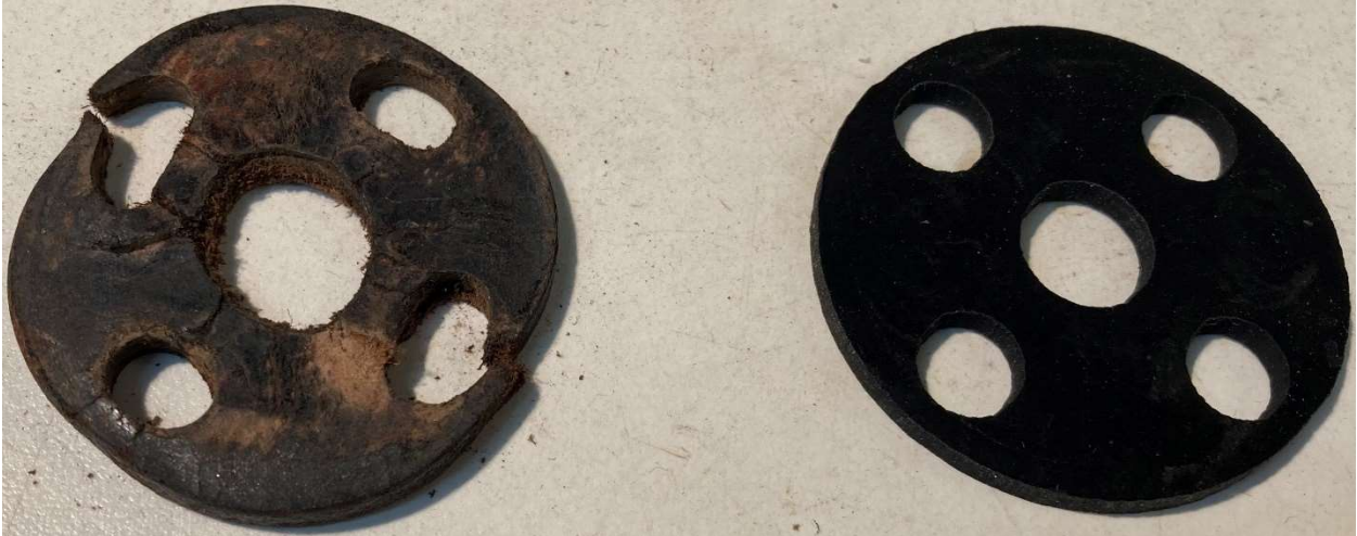
The old and new shock-absorbers for the motor-jointer connection.
