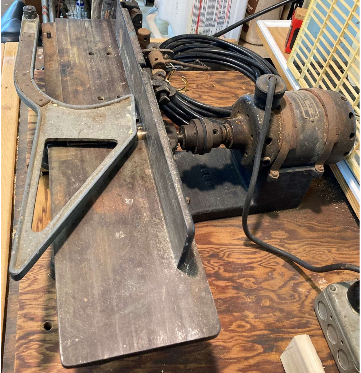
Crescent Machine Company Jointer manufactured about 1918
