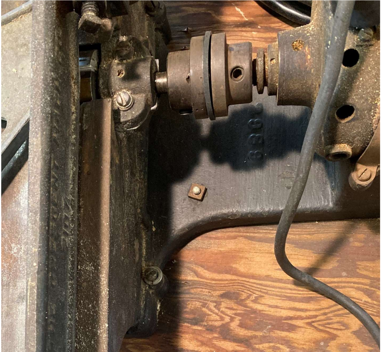
Fully cleaned up and reassembled, with the new shock-absorbing grommet in place.
