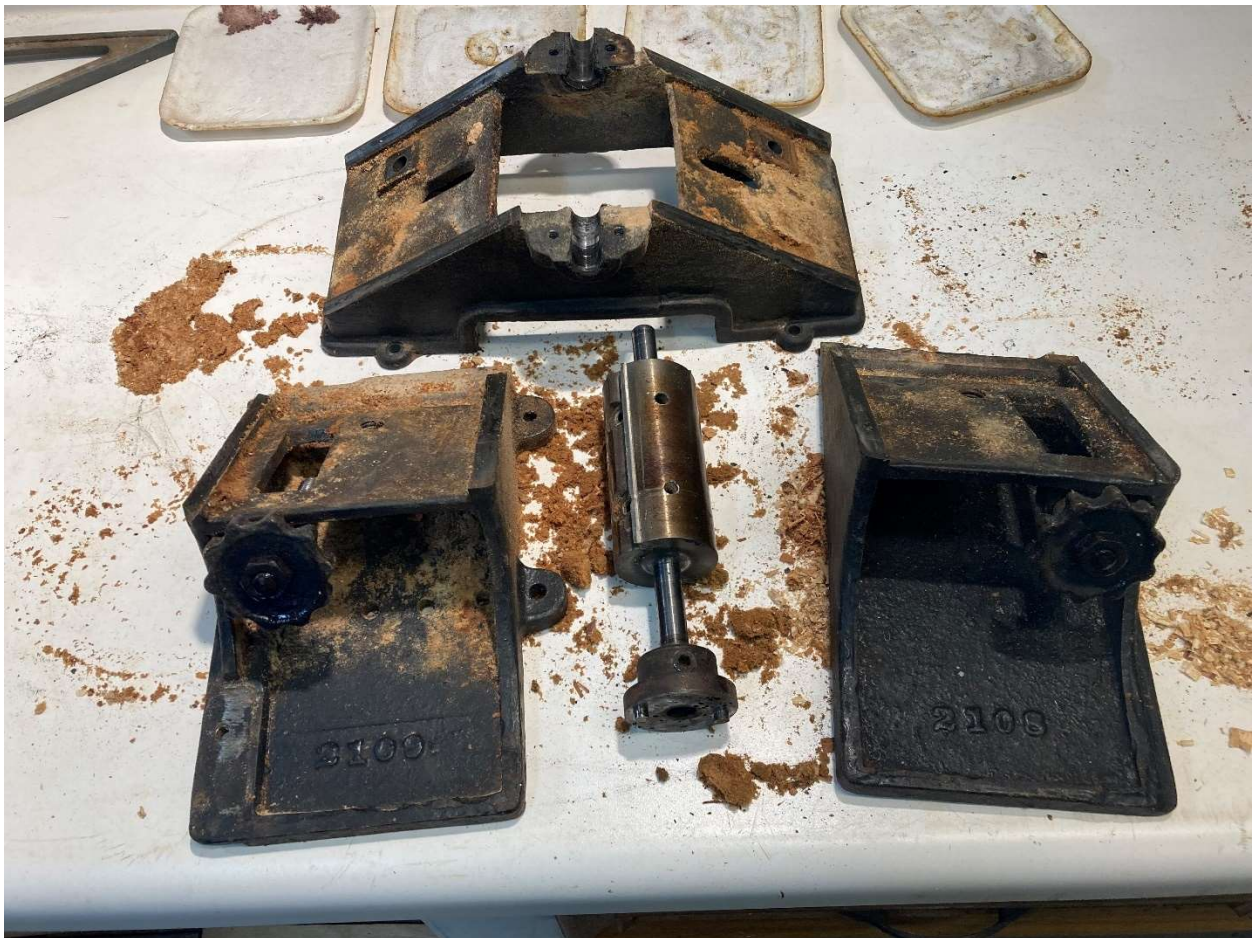
Disassembled except for the two slides, with most residue removed
