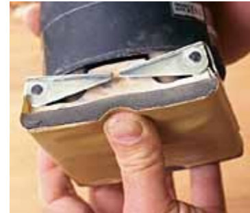
Soft backings on sanding tools won't support the sandpaper and make it cut more slowly.
