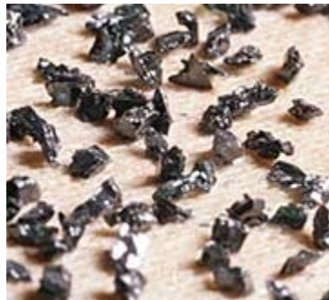
Abrasive grains are little sawteeth. This is 24-grit silicon carbide sandpaper before a size coat has been applied. It is easy to see how sharp the particles are.
