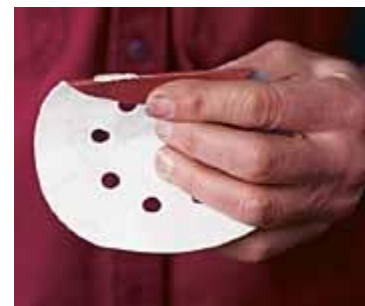
The adhesive and backing on a random-orbit sanding pad can crack if the disc is folded like ordinary sandpaper.
