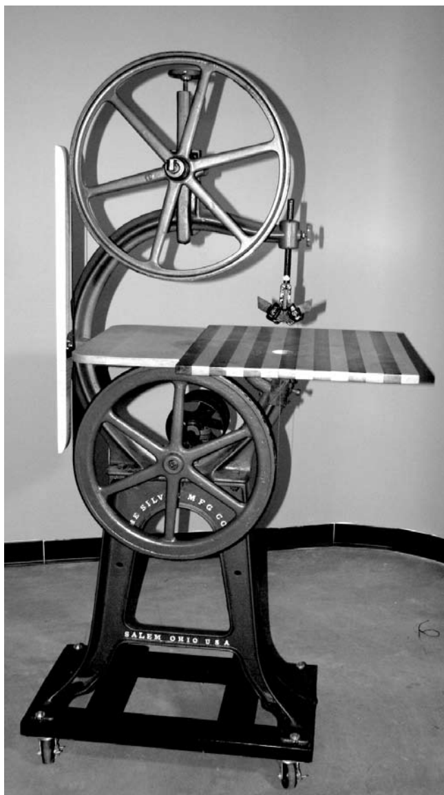
Figure 3. A circa 1897 20-inch Crescent band saw that is branded with the Silver Manufacturing Co. name cast into the base. OWNED AND RESTORED BY KEITH RUCKER.
