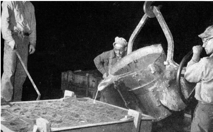
Figure 11. Crescent foundry workers pouring cast iron parts for Crescent Machines. IMAGE FROM THE 1946 CRESCENT CATALOG.
